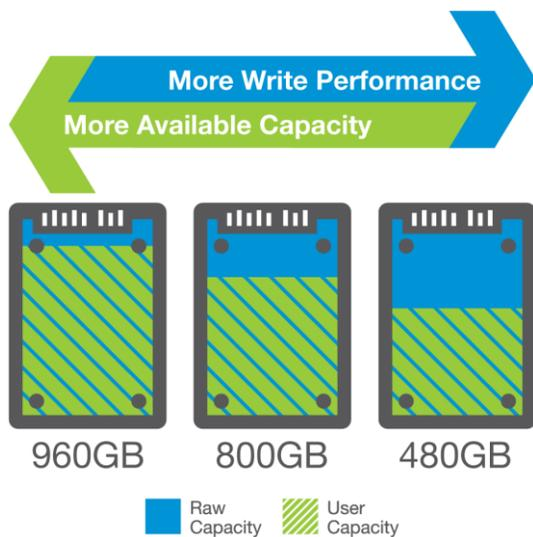
Figure 2: Flex Capacity Feature at Work
